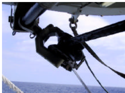
TufLine running through Odim Fairlead Tow Block
