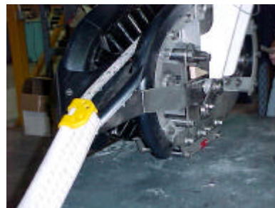
TufLine running through Odim Fairlead Tow Block
