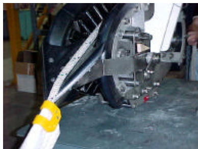
TufLine running through Odim Fairlead Tow Block
