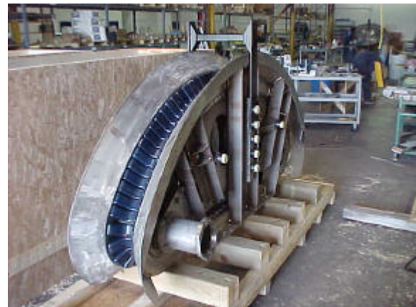
A Cable Overboarding Unit with 105 degree wrap angle undergoing 70 tonne static load testing.
